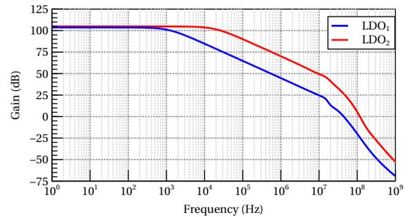
Fig. 6. Error Amplifier frequency response for both LDO regulators.
