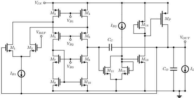
Fig. 5. High PSR LDO regulator using NMOS transistors in the EA differential pair.
