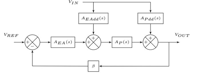
Fig. 3. LDO regulator block diagram for PSR analysis.
