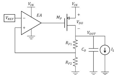
Fig. 2. Circuit diagram of typical LDO regulator.
