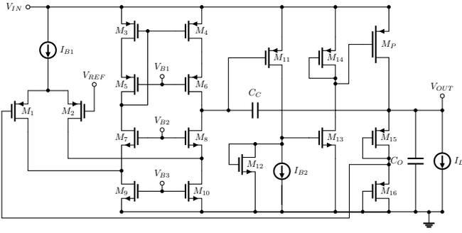
Fig. 4. High PSR LDO regulator using PMOS transistors in the EA differential pair.
