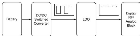
Fig. 1. Block diagram of a typical power management system used in SoCs.
